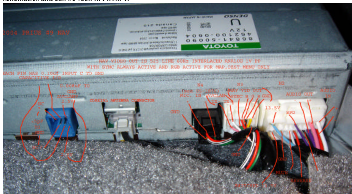
Photo 1 – back of navigation ECU under driver's seat
