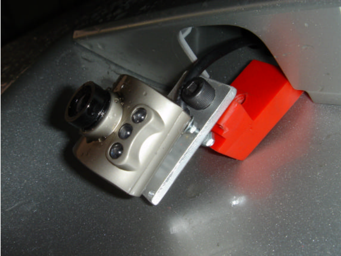
Photo 11– aluminum mounting plate for camera
